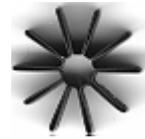
JFETs' temperature rise. The fins on the heat sink increase the surface area in contact with the air, increasing the thermal conductivity between the JFET and the air, thereby increasing the cooling. Mount the heat sink onto the JFET by pushing the case of the JFET into the hole in the center of the heat sink.
