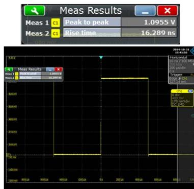
Fig. 3-5a: Properly compensated passive probe shows a nice, square wave. The peak-to-peak is about 1.09 volts and the rise time on that signal is about 16.2, 16.3 nanoseconds
