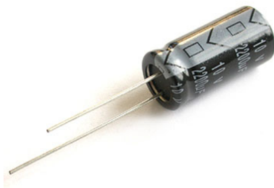
Radial Capacitor Negative lead on top
